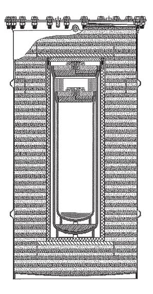
Figure 2-2. Conceptual cross-section of a 35-gallon DOT-certified shipping container.
